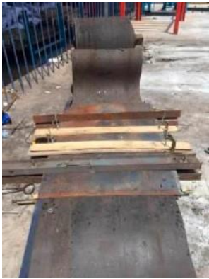
Finger splicing of monolayer bands.
